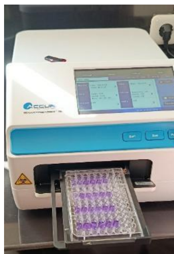
Figure 5. Measurement of Absorbance Values Using a Microplate Reader
