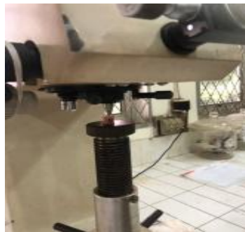
Figure 2. Surface hardness of the enamel test using the Vickers Hardness Tester
