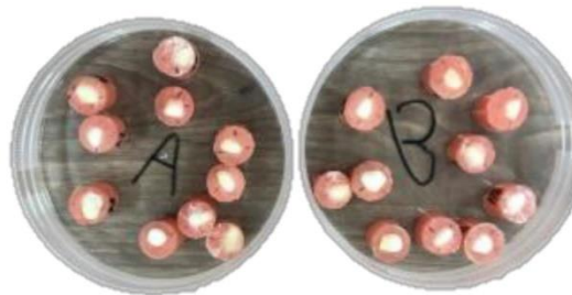
Figure 1. Samples placed in self-curing acrylic mould
